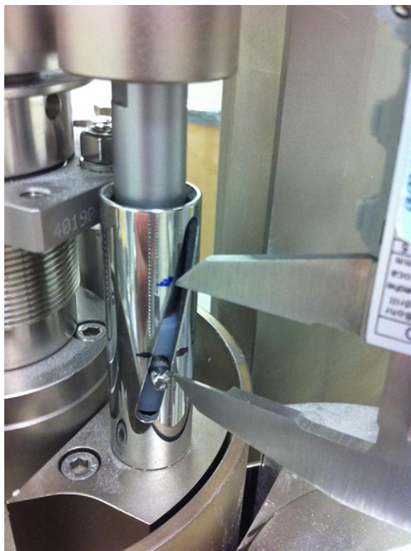
Fig. 1. Piston displacement measurement within a dosator.
