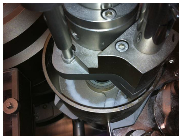
Fig. 4. Powder collapse during dosator movement due to formation of weak arches.
